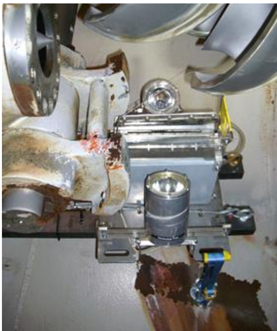
Pelton jet visualization at HPP Lünensee, VORARLBERGER ILLWERKE, Austria.
