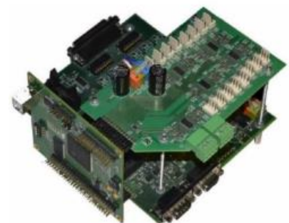
Control system with DSP TMS320F28335 + data acquisition extension.
