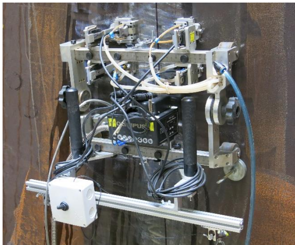
Scanning of welds – TOFD/PA testing.
