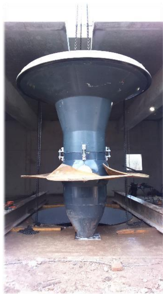
Vertical Kaplan Runner Ø 3,150 mm.
