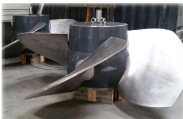
Axial Horizontal Kaplan Runner Ø 2,800 mm 2,000 kW.
