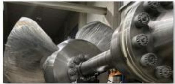
HEICO-TEC® Tension Nuts installed in main connection of turbine runner with main shaft.
