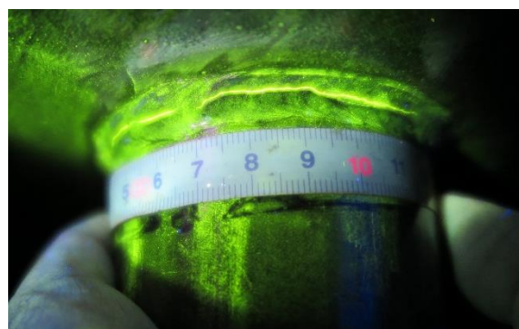
MT unacceptable indication in weld.
