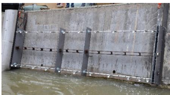
Current-meter measurements at HPP Erlabrunn, UNIPER, Germany.
