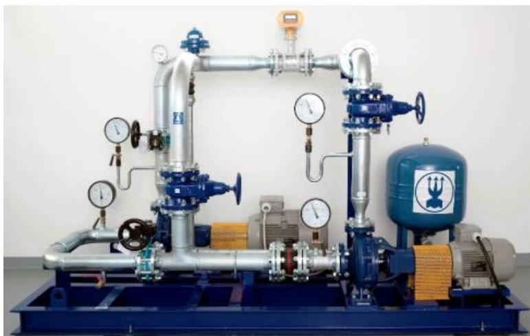
Small hydro power plant laboratory model.
