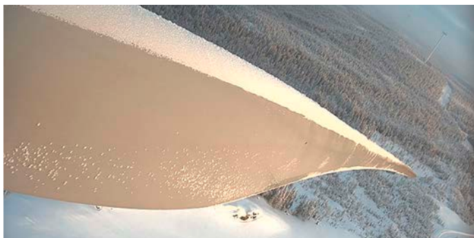
Ice build-up on a rotor blade
